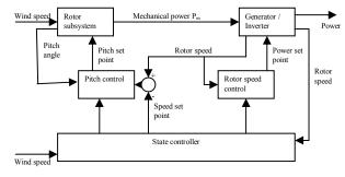
Figure 2: interactions between wind turbine's elements.
