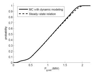
Figure 9: Cumulative distribution function of a 5 turbine wind farm generation obtained obtained with dynamic modeling and steady-state power curve with an annual mean wind speed of 10~m/s.
