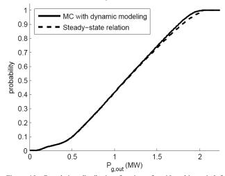
Figure 10: Cumulative distribution function of a 10 turbine wind farm generation obtained obtained with dynamic modeling and steady-state power curve with an annual mean wind speed of  $10~\rm m/s$ .
