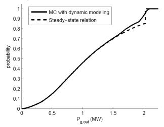
Figure 8: Cumulative distribution function of the wind turbine generation obtained with dynamic modeling and steady-state power curve with an annual mean wind speed of  $10.00 \, \text{m/s}$ .
