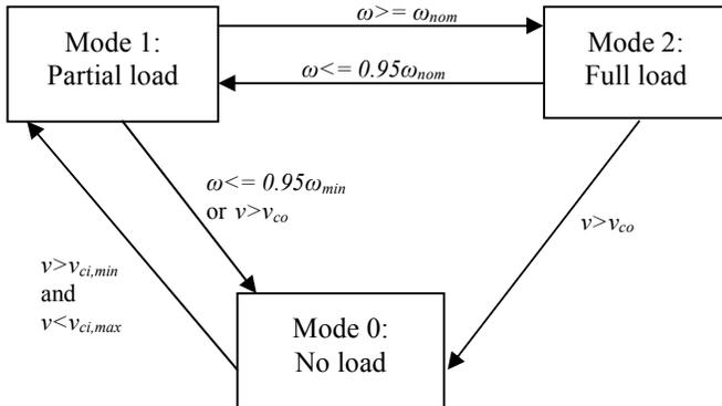
Figure 4: Control scheme of the variable speed DFIG wind turbine.
