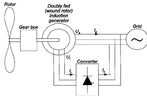
Figure 1: Connection of a DFIG wind turbine to the electrical network [16].
