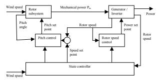
Figure 2: interactions between wind turbine's elements.
