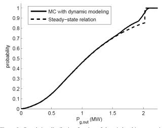
Figure 8: Cumulative distribution function of the wind turbine generation obtained with dynamic modeling and steady-state power curve with an annual mean wind speed of  $10~\rm m/s$ .
