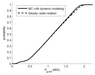
Figure 9: Cumulative distribution function of a 5 turbine wind farm generation obtained with dynamic modeling and steady-state power curve with an annual mean wind speed of  $10~\rm m/s$ .
