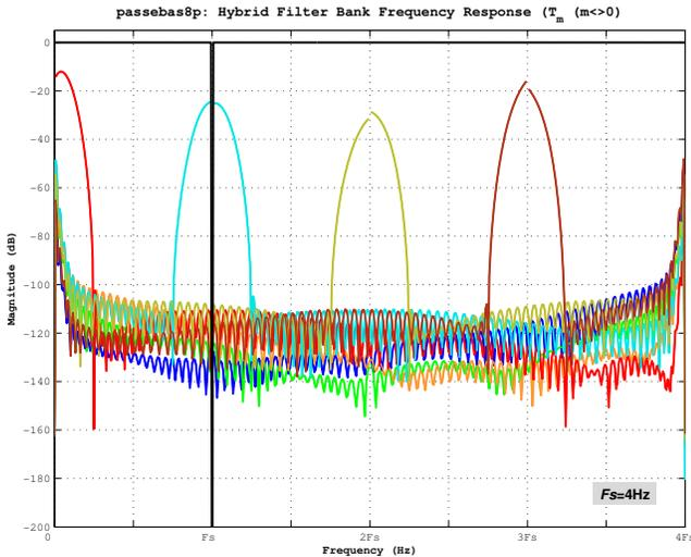
Fig. 5. Magnitude (dB) of the aliasing functions ( $m = 1, \dots, M-1$ ) for the whole band ( $|\omega| < \pi/T$ ).
