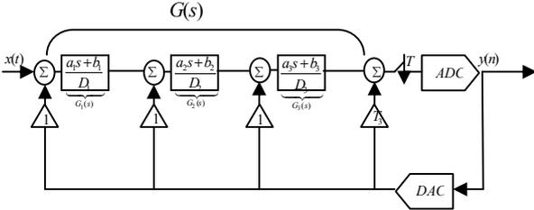
**Fig. 5.** Topology for a Continuous-time 6<sup>th</sup> order delta-sigma modulator.
