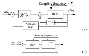
Figure 1: Single-bit CT (a) and DT (b) modulator
