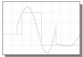
Figure 6: time domain simulations of the ADC input signal for CT, DT and ODT modulator.
