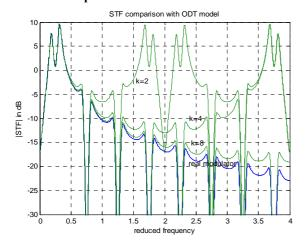
Figure 10: |STF| for k=2, 4, 8 for the ODT modulator compared with the CT modulator
