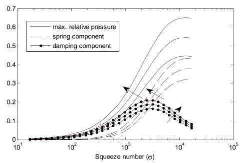
Fig. A-1 - influence of oscillation amplitude on small pressure hypothesis. As  $\alpha$  increases from 0.3 to 0.4, the different curves move in the direction of the arrows. The cutoff frequency and the domain of validity decrease with increasing  $\alpha$ .
