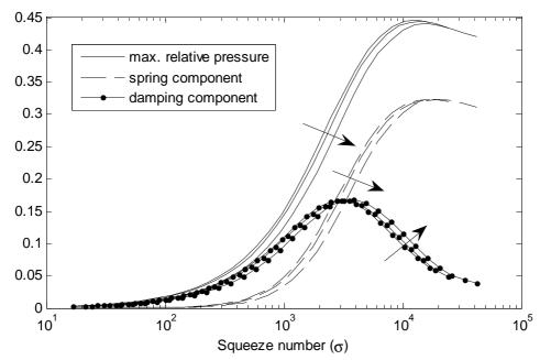
Fig. A-2 - influence of ambient pressure on small pressure hypothesis. As  $P_0$  decreases from  $10^5$  Pa to  $4 \times 10^4$  Pa, the different curves move in the direction of the arrows. The cutoff frequency and the domain of validity decrease with increasing  $P_0$ .
