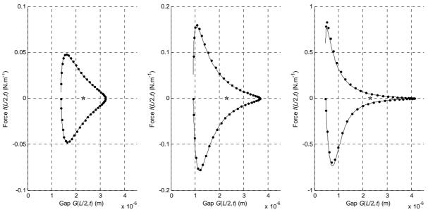
Fig. 1- Comparison of the finite difference model (dots) with the reduced-order model (continuous line). The results correspond, from left to right, to  $\alpha = 0.4$ ,  $\alpha = 0.6$  and  $\alpha = 0.8$ . The curves represent the value of the force per unit length at the middle of the bridge, i.e.  $f(L/2,t) = \int_0^W p(L/2,y,t) dy$ , versus  $G_\alpha(L/2,t)$ .
