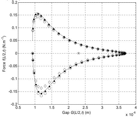
Fig. B-1 - Comparison of the finite difference model (continuous line) with three reducedorder models. The dots correspond to the reduced-order model presented in section II. The circles and the lozenges respectively correspond to the projection of (B-3) and (2) on an orthogonal basis verifying the boundary conditions.
