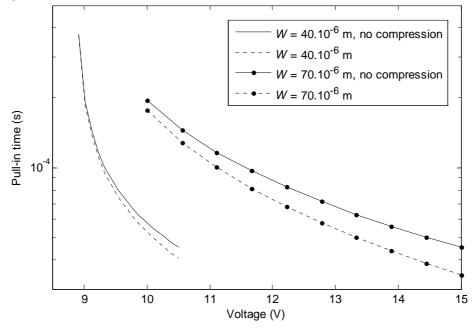
Fig. 6 – influence of compressibility on switching times, for  $P_0 = 1.013 \times 10^4$  Pa. The pull-in times calculated with our reduced-order model are represented for two different values of the width of the switch and compared to those obtained when neglecting compressibility.
