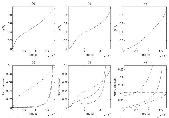
Fig. 5 – displacement of the midpoint of the switch vs. time (s), for  $P_0 = 1.013 \times 10^5$  Pa (a),  $P_0 = 1.013 \times 10^4$  Pa (b) and  $P_0 = 1.013 \times 10^3$  Pa (c) and V = 10 V. The displacement is normalized with respect to the gap. In the lower boxes, the corresponding fluidic pressure (continuous line) and electrostatic pressure (dashed line), normalized with respect to the ambient pressure,
