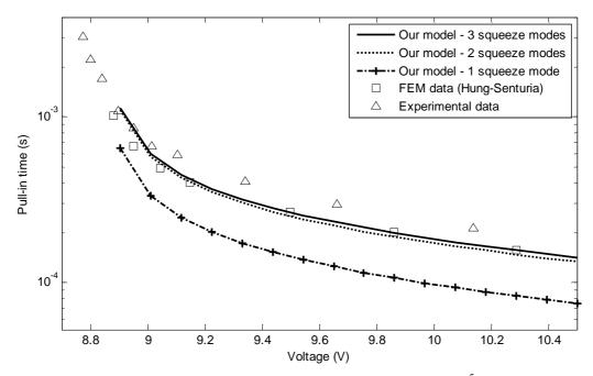
Fig. 2 - Pull-in time (s) versus applied voltage (V) for  $P_0 = 1.013 \times 10^5$  Pa. Comparison of the experimental and simulated results presented in [16] to the simulated results obtained with our reduced -order model. The chosen squeeze modes correspond to  $k_1 = 0$ , 1, 2 and  $k_2 = 1$  in (38). For the mechanical part, the first two eigenmodes are used.
