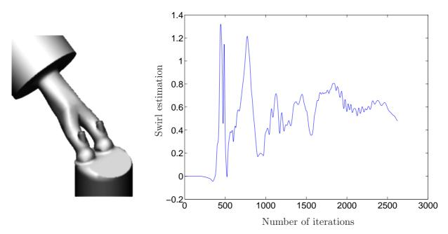
Figure 1: Simulation of airflow in an intake port of a Renault engine. This Navier-Stokes problem is solved iteratively by a finite element method. Left: 3D representation of an intake port. Right: value of the *swirl*, which quantifies the level of turbulence in the combustion chamber, as a function of the number of iterations of the solving procedure. Due to limitation of computer resources, the solver must be stopped before the stabilization of the solution.
