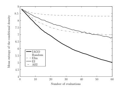
Figure 4: Convergence rates using EI, EIm, AEI, IAGO and random search, when convergence is measured by entropy of  $P_{X^*|\underline{\xi}_n}$ . The sample paths are simulated using the covariance (9) with  $\nu = 1.5$ ,  $\rho = 0.3$  and  $\sigma = 1.5$ . The standard deviation of noise is  $\sigma_N^2 = 0.5$ . We do not provide the convergence rates in terms of the distance to the maximum, as they are similar to those of Figure 3.
