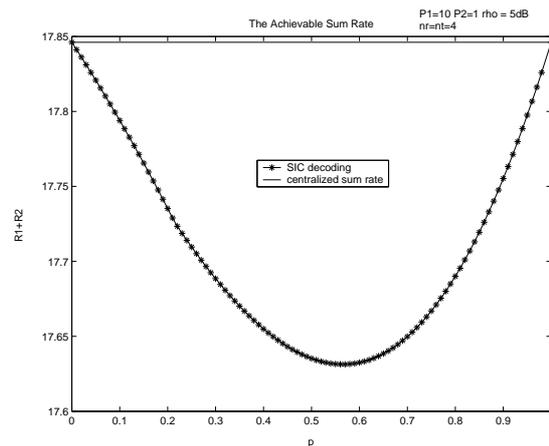
Figure 1: Temporal power allocation case. MAC sum-rate versus  $p$  for  $P_1 = 10$ ,  $P_2 = 1$ ,  $n_r = n_t = 4$ ,  $\rho = 5$  dB. The sum-rate of fading MIMO MACs is almost reached whatever the coordination signal distribution.
