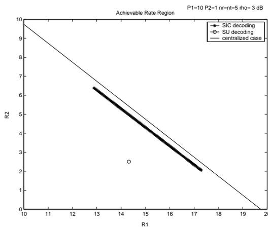
Figure 3: Achievable rate pairs for the **spatial** power allocation case for  $P_1 = 10$ ,  $P_2 = 1$ ,  $n_r = n_t = 5$ ,  $t_k = 0.2$ ,  $\rho = 3dB$ . The performance of the decentralized MAC with coordination is close to that of its centralized counterpart.
