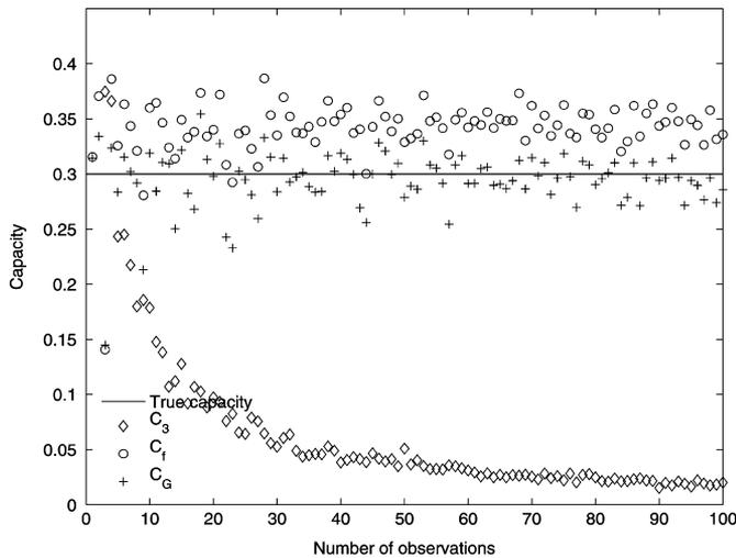
Fig. 4. Comparison of capacity estimators which worked for model (4) for increasing number of observations. Model (3) is used.  $\sigma^2 = 0.1$ ,  $n = 10$  receive antennas,  $m = 10$  transmit antennas. The rank of  $\mathbf{H}$  was 3.
