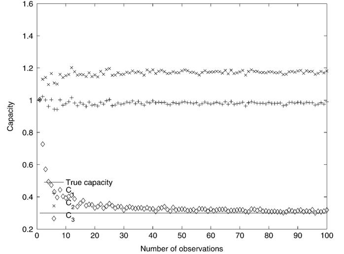
Fig. 1. Comparison of various classical capacity estimators for various number of observations, model (4).  $\sigma^2 = 0.1$ ,  $n = 10$  receive antennas,  $m = 10$  transmit antennas. The rank of  $\mathbf{H}$  was 3.
