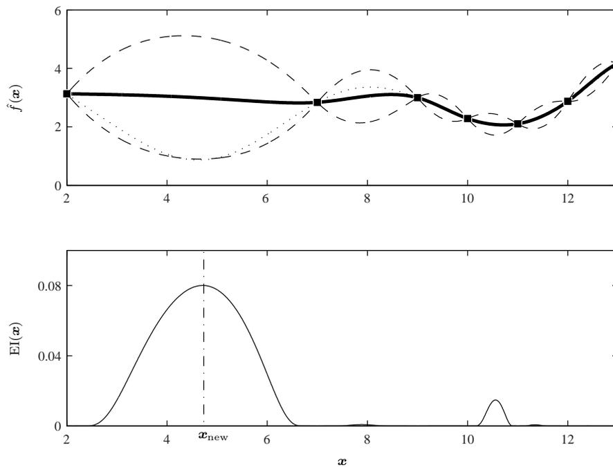
**Fig. 2** EI approach to optimization using Kriging: (*top*) prediction  $\hat{f}$  (bold line), 95% confidence intervals computed using  $\hat{\sigma}$  (dashed line) and true function  $f$  (dotted line); (*bottom*) expected improvement.
