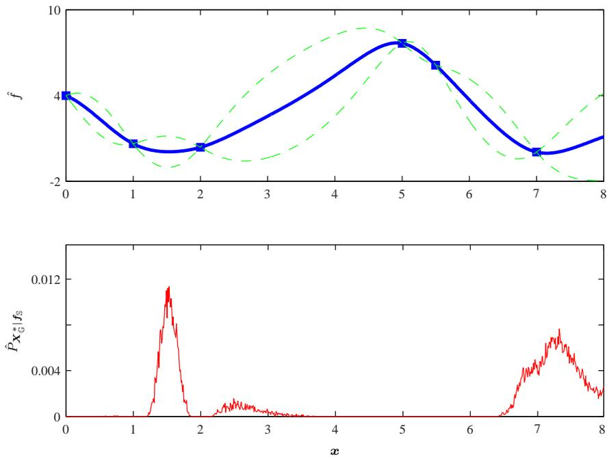
**Fig. 4** Estimation of the distribution of  $\mathbf{X}_{\mathbb{G}}^*$ : (top) Kriging interpolation, 95% confidence intervals and sample points; (bottom) estimated distribution of  $\mathbf{X}_{\mathbb{G}}^*$  using 10000 conditional simulations of  $F$  and a regular grid for  $\mathbb{G}$ .
