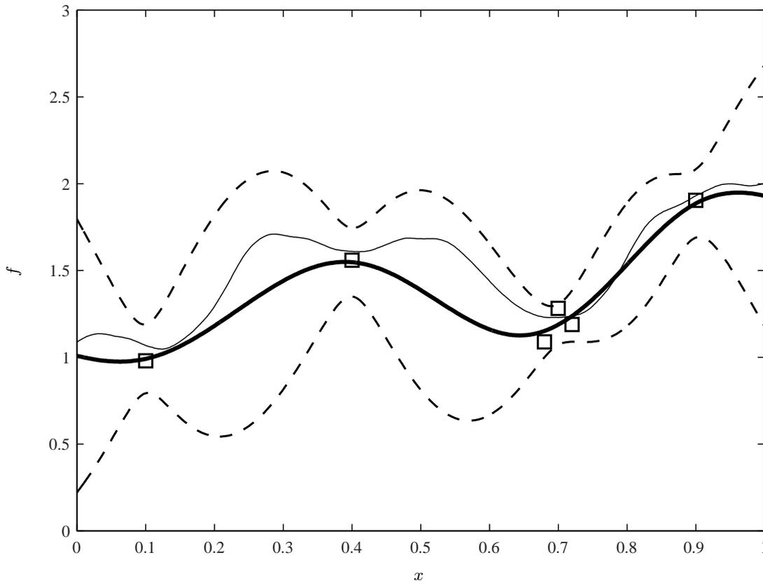
**Fig. 5** Example of prediction by Kriging (bold line) of noisy measurements represented by squares. Dashed lines represent 95% confidence regions for the prediction and the thin solid line is an example of conditional simulation obtained using the method presented in Section 5.3.1.
