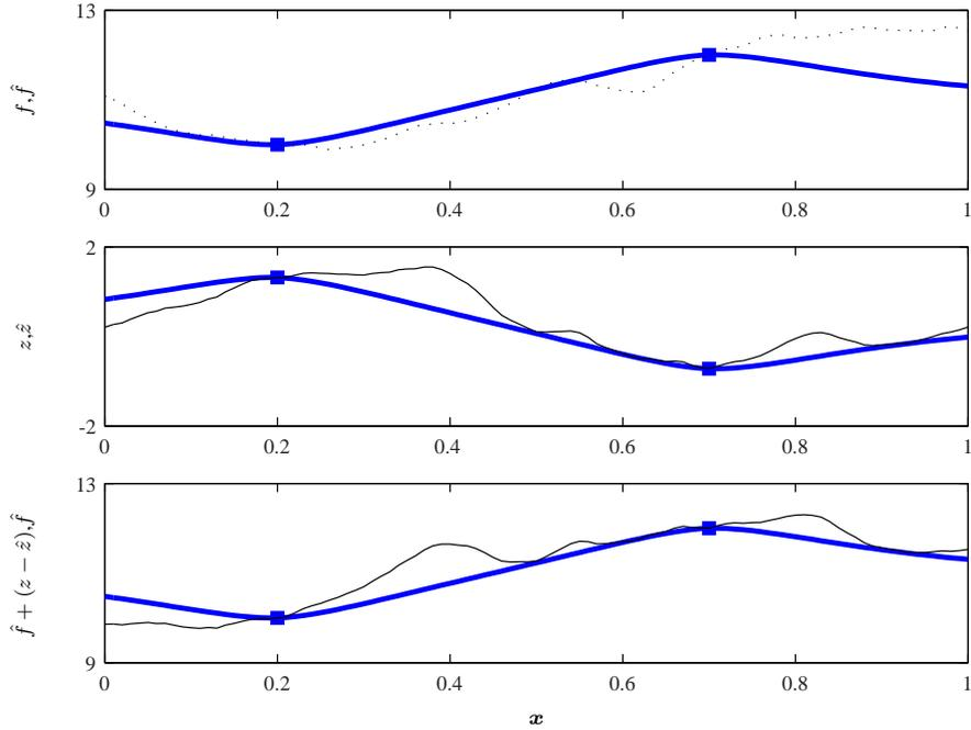
**Fig. 3** Conditioning a simulation: (*top*) unknown real curve  $f$  (dotted line), sample points (squares) and associated Kriging prediction  $\hat{f}$  (bold line); (*middle*) non-conditional simulation  $z$ , sample points and associated Kriging prediction  $\hat{z}$  (bold line); (*bottom*) the simulation of the Kriging error  $z - \hat{z}$  is picked up from the non-conditional simulation and added to the Kriging prediction to get the conditional simulation (thin line).
