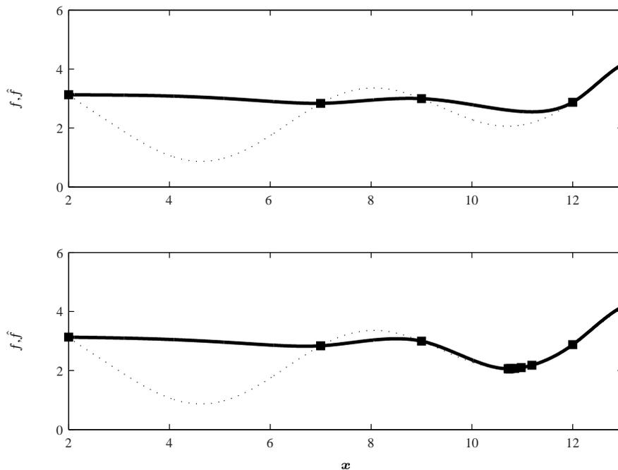
**Fig. 1** Naive approach to optimization using Kriging: (*top*) prediction  $\hat{f}$  (bold line) of the true function  $f$  (dotted line, supposedly unknown) obtained from an initial design materialized by squares; (*bottom*) prediction after seven iterations minimizing  $\hat{f}$ .
