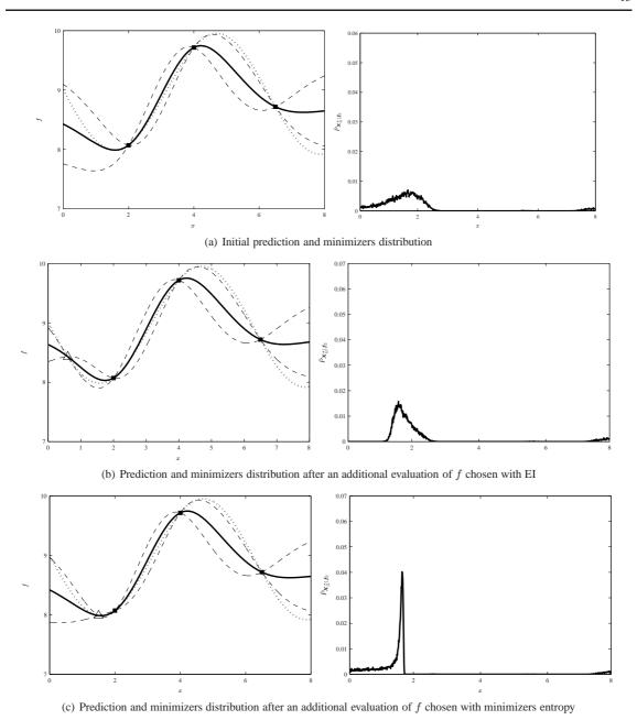
**Fig. 8** Comparison between minimizers entropy and EI: the *left* side contains the Kriging predictions before and after an additional evaluation chosen with either EI or minimizers entropy, while the *right* side presents the corresponding conditional distribution of the global minimizers.
