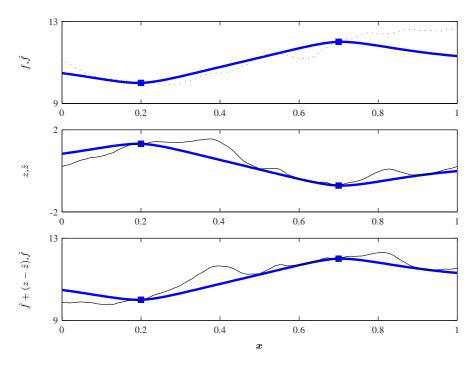
**Fig. 3** Conditioning a simulation: (top) unknown real curve f (doted line), sample points (squares) and associated Kriging prediction  $\hat{f}$  (bold line); (middle) non-conditional simulation z, sample points and associated Kriging prediction  $\hat{z}$  (bold line); (bottom) the simulation of the Kriging error  $z - \hat{z}$  is picked up from the non-conditional simulation and added to the Kriging prediction to get the conditional simulation (thin line).
