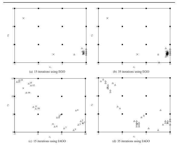
Fig. 9 Fifteen iterations of two optimization algorithms, that differ by their criteria for selecting evaluation points for f, on the Branin function: (top) the EI criterion is used, (bottom) the minimizers entropy criterion is used with a thousand candidate evaluation points for f set on a regular grid (squares account for initial data, triangles for new evaluations, and crosses give the actual locations of the three global minimizers).
