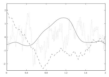
Fig. 11 Three sample paths of a zero-mean Gaussian process with a Matérn covariance. Conventions are as in Figure 10:  $\nu=4$  for the solid line,  $\nu=1$  for the dashed line and  $\nu=0.25$  for the dotted line.
