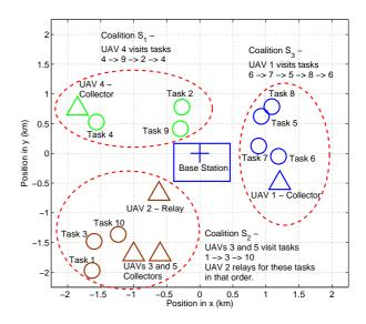
Fig. 3. A snapshot of a final coalition structure resulting from the proposed hedonic coalition formation algorithm for a network of  $M=5\,$  UAVs and  $T=10\,$  tasks.
