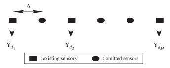
**Fig. 1.** Example of NLA and its equivalent ULA, with  $\mathbf{d} = [0, 2, 5]\lambda/2$ , i.e.  $c_1 = 0$ ,  $c_2 = 2$  and  $c_3 = 5$ .
