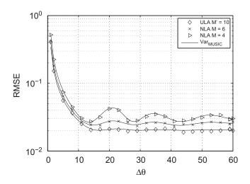
**Fig. 7.** RMS error for the source at  $0^{\circ}$  with ULA M' = 10 and NLAs with M = 6 and 4 respectively, at SNR = 10 dB, N = 2 sources.
