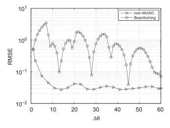
**Fig. 8.** RMS error for the source at  $0^{\circ}$  with NLA M = 4 using root-MUSIC and beamforming, at SNR = 10 dB, N = 2 sources.
