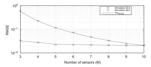
**Fig. 4.** RMS error for the source at  $-5^{\circ}$  with M = 3, 4, ..., 10, SNR = 10 dB, DOA =  $[-5^{\circ}, 10^{\circ}]$  in the case of ULA and NLA.
