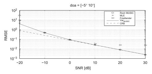
**Fig. 3.** RMS error for the source at  $10^{\circ}$  for the array  $\mathbf{d} = [0, 1, 3, 6, 9]\lambda/2$ , DOA =  $[-5^{\circ}, 10^{\circ}]$ .
