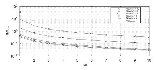
**Fig. 6.** Resolution for the source at  $0^{\circ}$  with M' = 10, 6 and 4 in the case of ULA, M = 6 and 4 in the case of NLA, at SNR = 10 dB, N = 2 sources.
