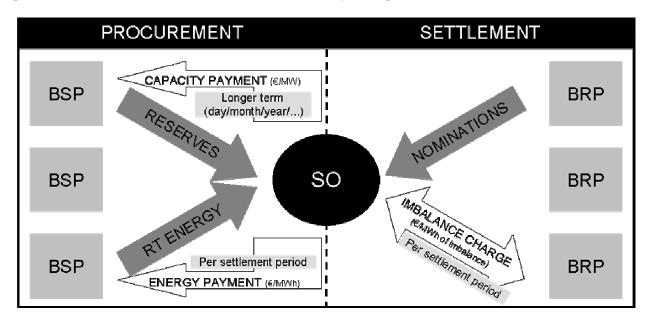
Figure 1: Balancing services procurement and imbalance settlement by SO
