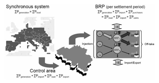
Figure 2: SO versus BRP responsibility in the synchronous area UCTE
