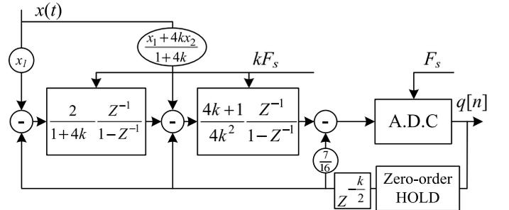
Fig. 8. Equivalent  $2^{nd}$  order ODT  $\Sigma\Delta$  modulator
