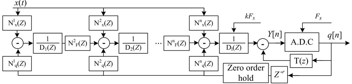
Fig. 18. ODT topology for simulation
