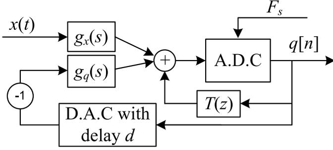
Fig. 4. CT  $\Sigma\Delta$  modulator
