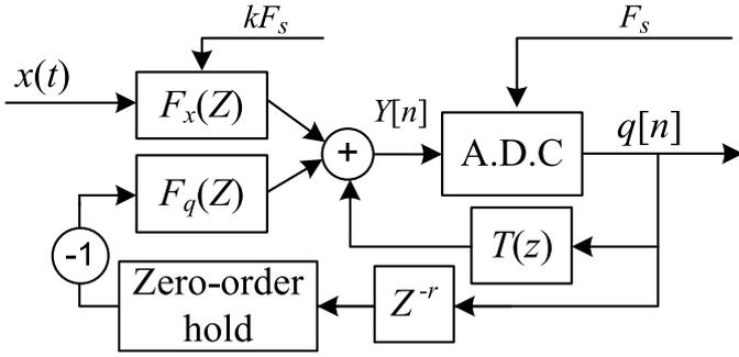
Fig. 5. ODT  $\Sigma\Delta$  modulator
