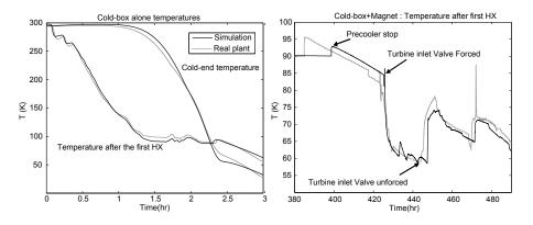
Figure 8: Comparison between experimental and simulated temperatures during a cool-down of the cold box alone and with the CMS magnet
