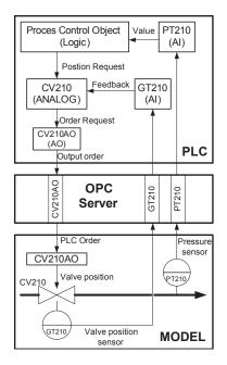
Figure 2: Links between the PLC and the process model
