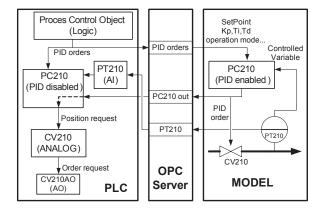
Figure 3: PID controller management in simulator
