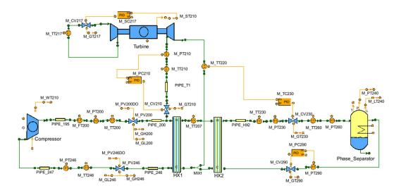
Figure 5: Small cryogenic model overview in EcosimPro
