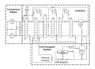
Figure 7: The CMS cryoplant
