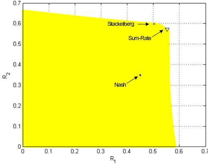
Fig. 7. Achievable rate region for the inter-operator spectrum sharing game. Both operators achieve better payoffs when adopting the hierarchical (Stackelbeg) approach.
