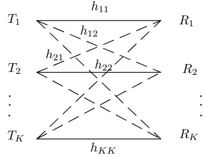
Fig. 1. K-Transmitters N-Carriers interference channel under study. is characterized by its received noise power on each carrier  $n$ , by  $\sigma_n^2$ .
