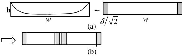
Fig. 3. (a). The skin effect leads to non-homogeneous flux distribution in magnets. This can be modeled by two bands with homogeneous flux. (b). Segmentation doubles number of bands, as well as eddy-current losses.
