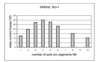
Fig. 5. Variation of the eddy-current losses with respect to number of pole arc magnet segments at f=5400Hz and with only one segment in Z direction.
