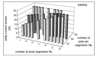
Fig. 6. Variation of the eddy-current losses with respect to number of pole arc and of axial magnet segments, at f=5400Hz
