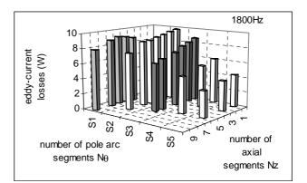
Fig. 8. Variation of the eddy-current losses with respect to number of pole arc and of axial magnet segments, at f=1800Hz
