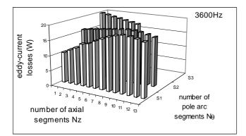
Fig. 7. Variation of the eddy-current losses with respect to number of pole arc and of axial magnet segments, at f=3600Hz
