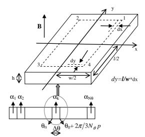
Fig. 1. Cross section of one pole magnet and one of its segmentation
