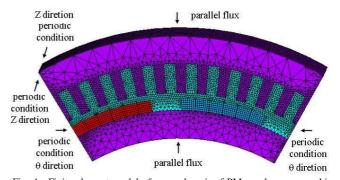
Fig. 4. Finite element model of one pole-pair of PM synchronous machine, with 6 PM segments in circumferential direction and 10 in axial direction. The dimension in Z direction of this model corresponds to 1/10 of the entire machine length, i.e. 250/10=25mm.
