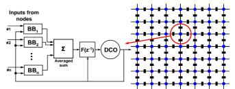
Figure 4. The proposed ADPLL network. DCO stands for Digital-Controled oscilaltor, F the filter, BB the bang-bang phase detector.
