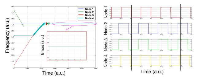
Figure 8. Simulation results on a 2x2 network with a symetric comparison strategy: frequency of the nodes and a zoom on their errors with the master clock (left), temporel signal in steady state of each generated clock (right)
