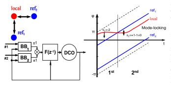
Figure 6. Node without assymetric comparison strategy, mode-locking
