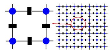
Figure 1. Active clock distribution network
