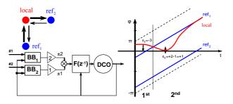
Figure 7. Node with assymetric comparison strategy, mode-locking avoidance
