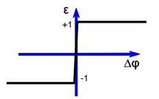
Figure 5. Bang-bang phase detector static response in phase domain
