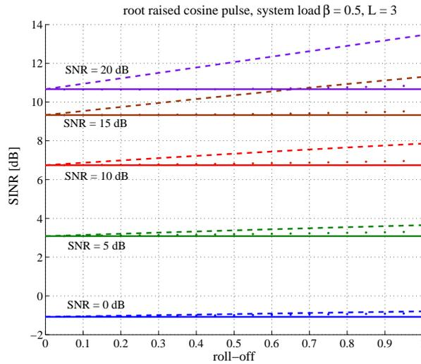
Fig. 4. Asymptotic output SINR of a multistage Wiener filter with  $L = 3$  versus the roll-off  $\theta$  as front-end A (dashed lines) and front-end B (dots) are in use in an asynchronous CDMA system. The solid lines show the reference performance in synchronous CDMA systems. The curves are parametric in the input SNR with SNR varying between 0 dB and 20 dB in steps of 5 dB.
