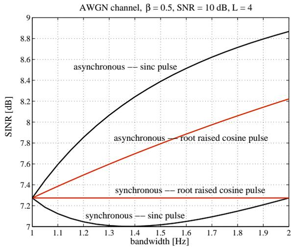
Fig. 2. Output SINR of a multistage Wiener filter with  $L = 4$  versus bandwidth. CDMA systems with equal received powers, root raised cosine chip waveforms or sinc pulses, system load  $\beta = \frac{1}{2}$  and input SNR = 10 dB are considered.
