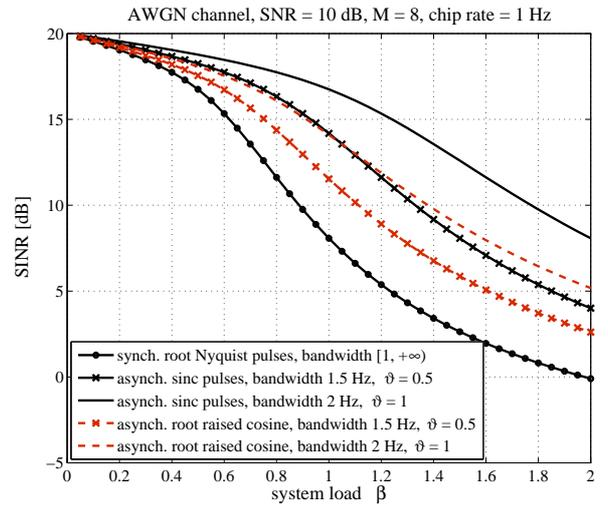
Fig. 3. Output SINR of a multistage Wiener filter with  $L = 8$  versus the system load. Asynchronous CDMA systems with equal received powers, root raised cosine chip waveforms or sinc pulses with bandwidth  $B = 1.5, 2$  Hz, input SNR = 10 dB are compared to synchronous CDMA systems with root Nyquist chip pulses.
