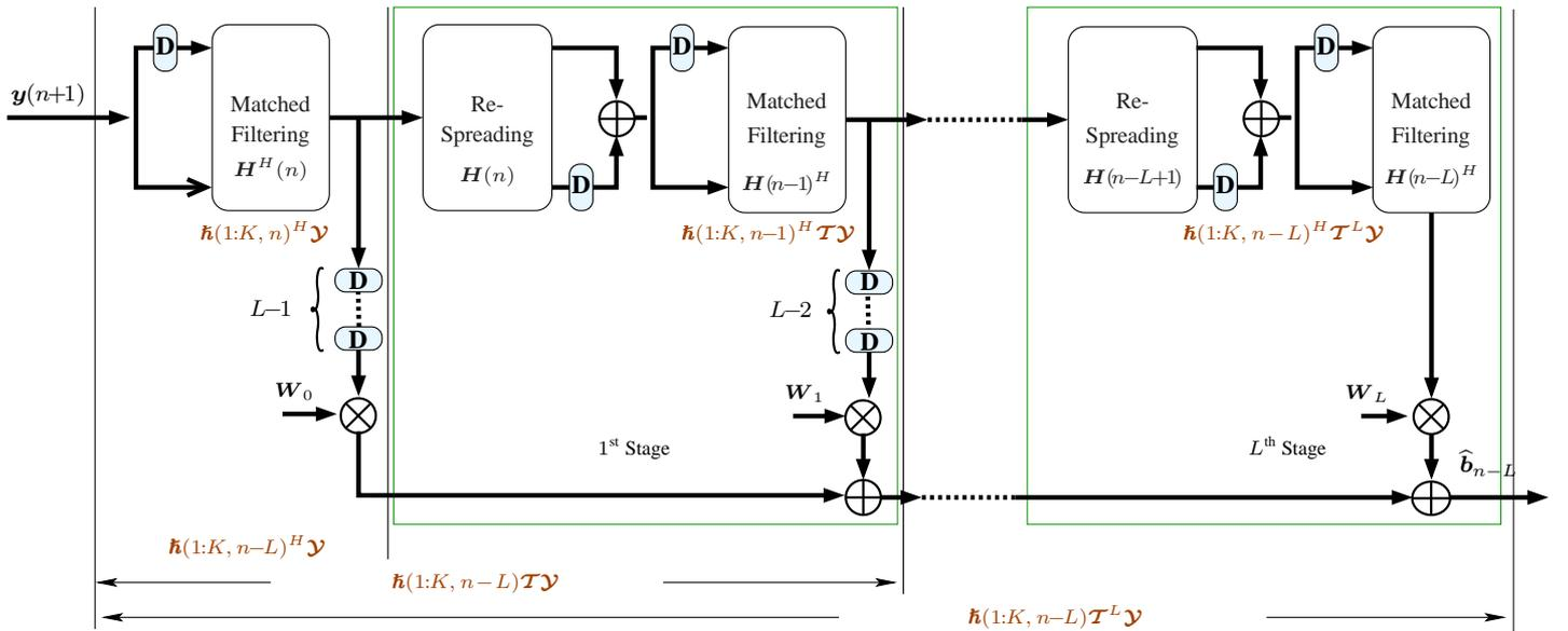
Fig. 1. Multistage detector for asynchronous CDMA systems. Here,  $\tilde{\mathbf{h}}(1:K, n) = [\Phi_1 \mathbf{s}_1^{(n)}, \Phi_2 \mathbf{s}_2^{(n)}, \dots, \Phi_K \mathbf{s}_K^{(n)}]$
