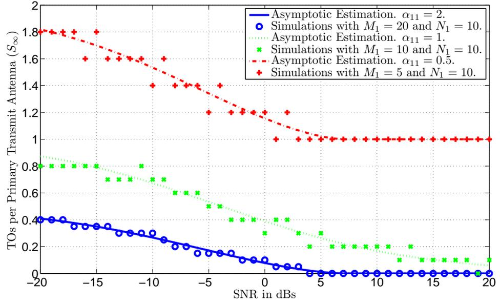
Figure 2. Fraction of transmit opportunities in the RLNA (Def. 4), i.e.,  $S_\infty$  (27) as function of the SNR =  $\frac{p_{1,\max}}{\sigma_1^2}$  and  $\alpha_{11} = \frac{M_1}{N_1}$ . Simulation results are obtained by using one realization of the matrix  $\mathbf{H}_{11}$  when  $N_1 = 10$ .
