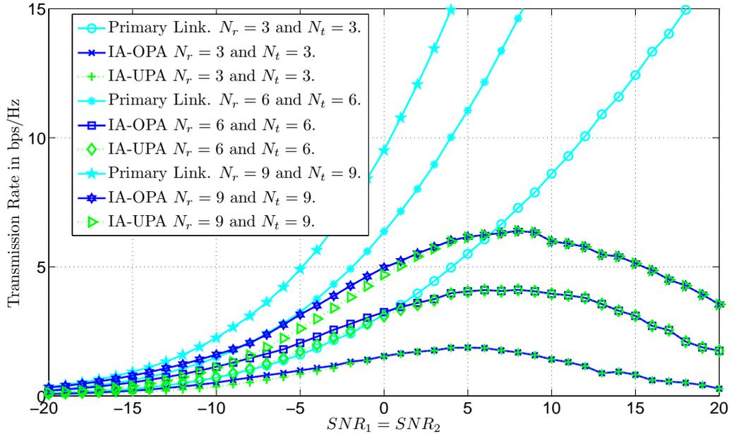
Figure 4. Transmission rate of the opportunistic link obtained by Monte Carlo simulations as a function of the  $SNR_1 = SNR_2$ . The number of antennas satisfy  $M_1 = M_2 = N_t$  and  $N_1 = N_2 = N_r$ , with  $N_t = N_r$ , and  $N_r \in \{3, 6, 9\}$  and  $SNR_i = \frac{p_{i,\max}}{\sigma_i^2}$ , for all  $i \in \{1, 2\}$ .
