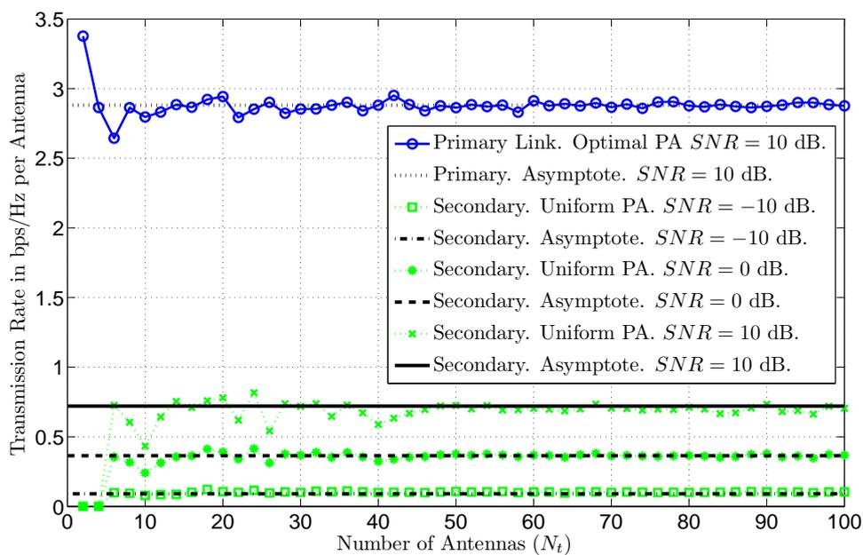
Figure 6. Asymptotic transmission rates per antenna of the opportunistic link as a function of the number of antennas when  $N_r = N_t$  using uniform PA at different SNR levels  $\text{SNR}_i = \frac{p_{i,\max}}{\sigma_i^2}$ . Simulation results are obtained using one channel realization for matrices  $\mathbf{H}_{ij} \forall (i, j) \in \{1, 2\}^2$  and theoretical results using Prop. 5,
