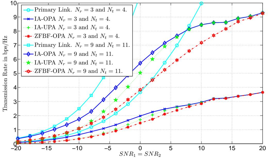
Figure 3. Transmission rate of the opportunistic link obtained by Monte Carlo simulations as a function of the  $\text{SNR}_1 = \text{SNR}_2$  when IA and ZFBF are implemented. The number of antennas satisfy  $\alpha = \frac{N_t}{N_r} \approx \frac{5}{4}$ , with  $M_1 = M_2 = N_t$  and  $N_1 = N_2 = N_r \in \{3, 9\}$  and  $\text{SNR}_i = \frac{P_i^{\max}}{\sigma_i^2}$ , for all  $i \in \{1, 2\}$ .
