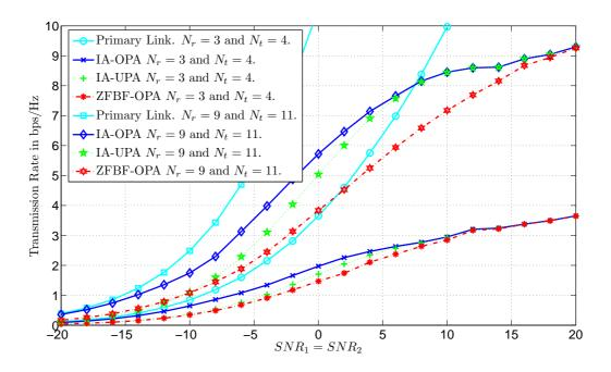
Figure 3. Transmission rate of the opportunistic link obtained by Monte Carlo simulations as a function of the SNR<sub>1</sub> = SNR<sub>2</sub> when IA and ZFBF are implemented. The number of antennas satisfy  $\alpha = \frac{N_t}{N_r} \approx \frac{5}{4}$ , with  $M_1 = M_2 = N_t$  and  $N_1 = N_2 = N_r \in \{3, 9\}$  and SNR<sub>i</sub> =  $\frac{p_{i,\max}}{\sigma_1^2}$ , for all  $i \in \{1, 2\}$ .
