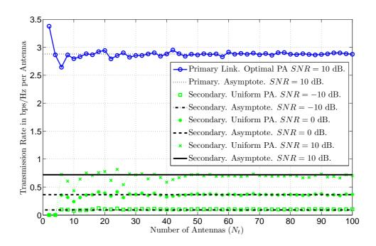
Figure 6. Asymptotic transmission rates per antenna of the opportunistic link as a function of the number of antennas when  $N_r = N_t$  using uniform PA at different SNR levels  $\text{SNR}_i = \frac{p_{i,\max}}{\sigma_i^2}$ . Simulation results are obtained using one channel realization for matrices  $\mathbf{H}_{ij} \ \forall (i,j) \in \{1,2\}^2$  and theoretical results using Prop. 5,
