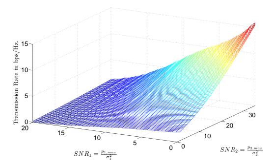
Figure 5. Transmission rate of the opportunistic link obtained by Monte Carlo simulations as a function of the  $SNR_i = \frac{p_{i,max}}{\sigma_i^2}$ , with  $i \in \{1, 2\}$ . The number of antennas satisfy  $M_1 = M_2 = N_t$  and  $N_1 = N_2 = N_r$ , with  $N_r = N_t = 4$ .
