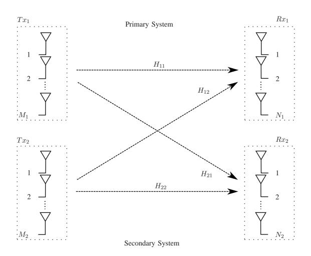
Figure 1. Two-user MIMO interference channel.
