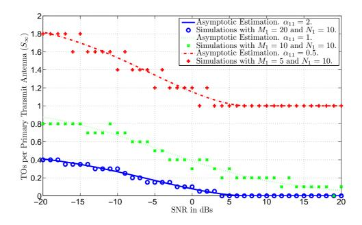
Figure 2. Fraction of transmit opportunities in the RLNA (Def. 4), i.e.,  $S_{\infty}$  (27) as function of the SNR =  $\frac{p_{1,\text{max}}}{\sigma_1^2}$  and  $\alpha_{11} = \frac{M_1}{N_1}$ . Simulation results are obtained by using one realization of the matrix  $\mathbf{H}_{11}$  when  $N_1 = 10$ .
