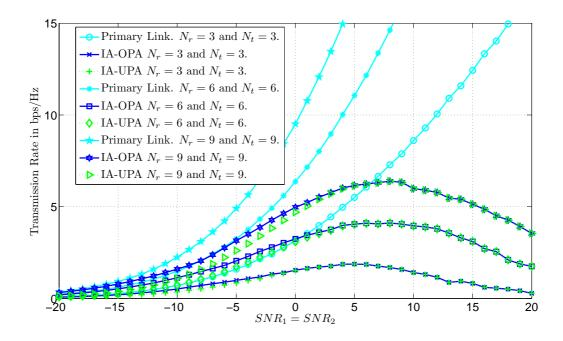
Figure 4. Transmission rate of the opportunistic link obtained by Monte Carlo simulations as a function of the SNR<sub>1</sub> = SNR<sub>2</sub>. The number of antennas satisfy  $M_1 = M_2 = N_t$  and  $N_1 = N_2 = N_r$ , with  $N_t = N_r$ , and  $N_r \in \{3, 6, 9\}$  and SNR<sub>i</sub> =  $\frac{p_{i,\text{max}}}{\sigma_i^2}$ , for all  $i \in \{1, 2\}$ .
