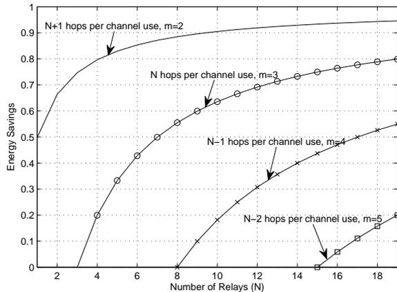
Fig. 1. The average energy savings curves versus the number of relays, using the distributed protocols for cooperative routing with distributed space-time codes of  $m$  cooperating nodes when the end-to-end outage probability is  $\rho_{\max} = 10^{-4}$ .
