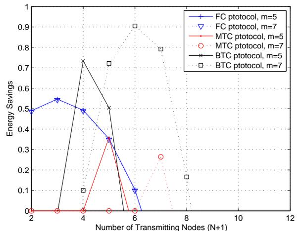
Fig. 2. The average energy savings curves versus the number of relays, using the distributed power allocation for cooperative routing with distributed space-time codes of  $m$  cooperating nodes when per hop outage probability requirement is  $\rho_0 = 10^{-5}$ .
