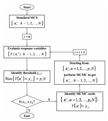
Fig. 1.1. Sketch of the SS algorithm
