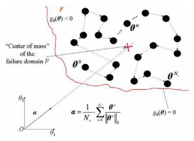
**Fig. 1.4.** Line Sampling important unit vector  $\alpha$  taken as the normalized "center of mass" of the failure domain *F* in the standard normal space. The "center of mass" of *F* is computed as an average of *N*<sub>s</sub> failure points generated by means of a Markov chain starting from an initial failure point  $\theta^0$  (Koutsourelakis et al. 2004)
