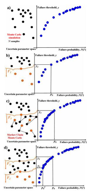
**Fig. 1.2.** Illustration of the SS procedure: a) Conditional level 0: Standard Monte Carlo simulation; b) Conditional level 0: adaptive selection of  $y_1$ ; c) Conditional level 1: Markov Chain Monte Carlo simulation; d) Conditional level 1: adaptive selection of  $y_2$  (Au 2005)
