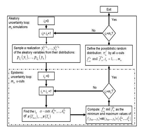
Figure 2: The hybrid method for uncertainty propagation
