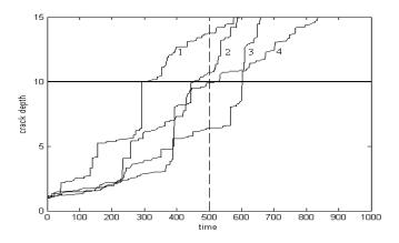
Figure 4: Four different realizations of degradation evolution
