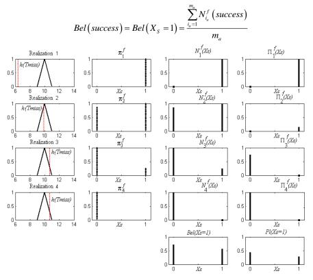
**Figure 5:** Application of the hybrid method of uncertainty representation (columns 1-2) and joint aggregation method for the uncertainty propagation (column 3-4), with regards to the four realizations of the degradation process shown in Figure 4
