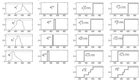
**Figure 10:** Application of the hybrid method of uncertainty representation (column 1) and Ferson aggregation method for the uncertainty propagation (columns 2-4), with regards to the four realizations of the degradation process shown in Figure 4.
