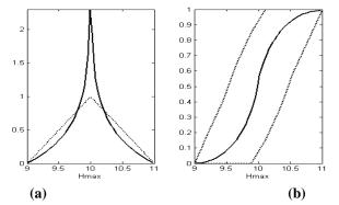
**Figure 3:** (a) Possibilistic distribution of  $H_{\text{max}}$  (dotted line) and its probabilistic transformation (continuous line); (b) corresponding necessity and possibility measures of the set  $(-\infty, H_{\text{max}}]$  (dotted line) and cumulative distribution function of  $H_{\text{max}}$  considered by the purely probabilistic method (continuous line).
