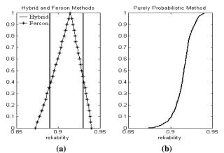
**Figure 7:** Comparison of the results obtained with: (a) joint aggregation method (continuous line), Ferson aggregation method (asterisk) and (b) purely probabilistic method
