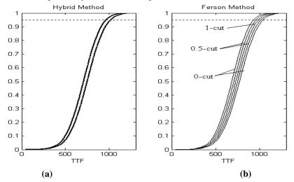
Figure 9: Comparison of the results obtained with: (a) joint aggregation method, (b) Ferson aggregation method
