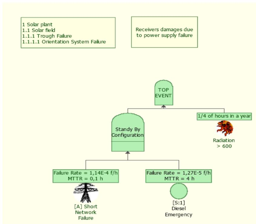
where the failure rate and the mean time to repair (MTTR) of the ‘Diesel Emergency’ event are given by the following FT
