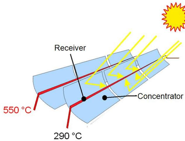
Figure 2: parabolic solar collectors
