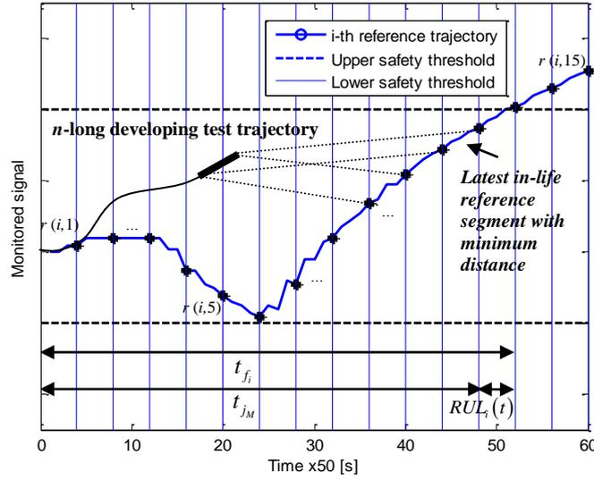
**Figure 6** The remaining time before failure  $RUL_i(t)$  on the reference trajectory of Figure 2 starting from the end time of the latest-in-life segment of minimum distance from the occurring trajectory
