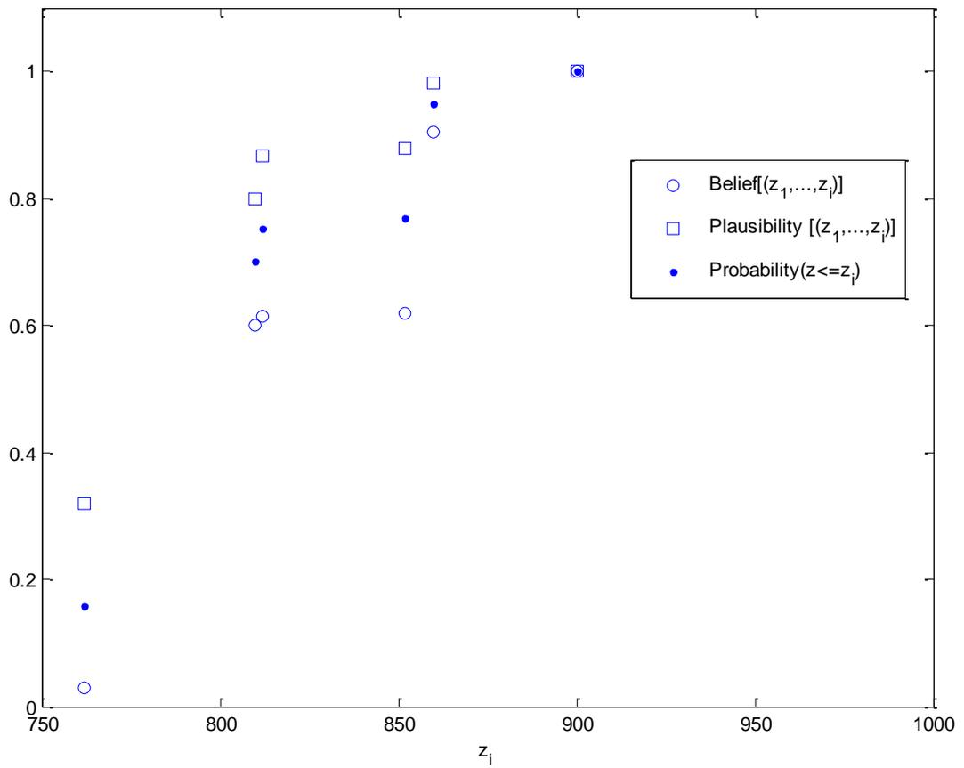
**Figure 5. Belief (circles), plausibility (squares) of the sets  $[z_1, \dots, z_i]$  obtained by the DST approach and cumulative density probability values (dots) obtained by the Bayesian approach.**
