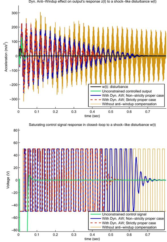
Fig. 3. Comparison of the anti-windup closed-loop behavior responses
