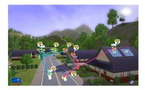
**Fig. 1**. Dense rechargeable base stations which coordinate their transmissions towards users by forming reconfigurable virtual antenna arrays.
