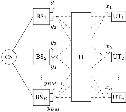
Fig. 1. Schematic system model for the case  $M = 2$ .
