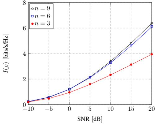
Fig. 3. Ergodic mutual information  $I(\rho)$  versus SNR. Markers indicate simulation results, solid lines correspond to the deterministic equivalent approximation  $V(\rho)$  as given by Theorem 1 (ii).
