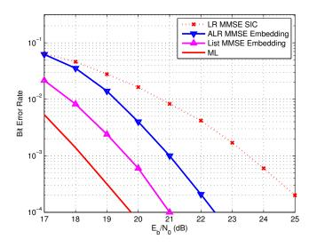
Figure 1. Bit error rate vs. average SNR per bit for the uncoded  $10 \times 10$  system using 64-QAM.
