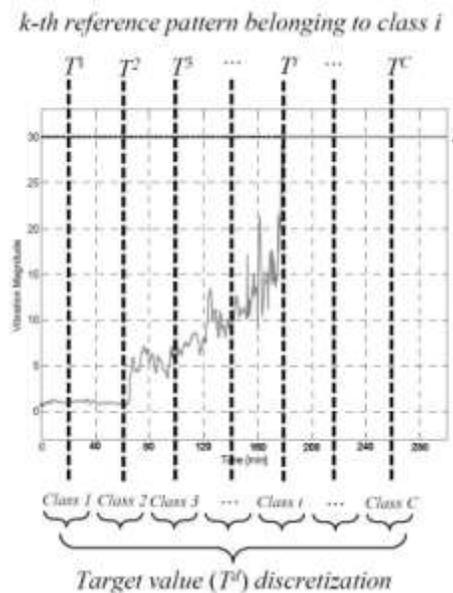
Figure 7. schematic sketch of the class discretization
