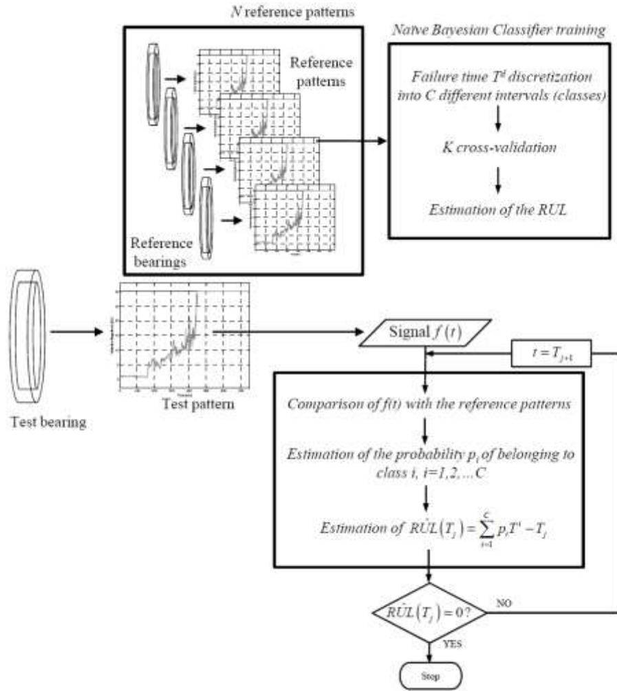
Figure 6. schematic sketch of the computational framework
