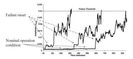
Figure 1. Typical behavior of degraded bearings measurements [8]
