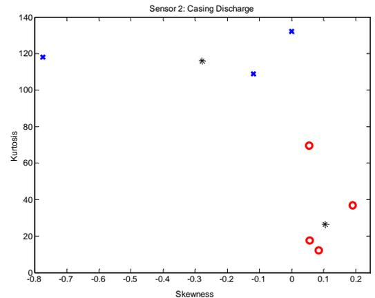
Figure 10. Classification results for sensor S2 (Classifier 2). Circles = Healthy, Crosses = Failed
