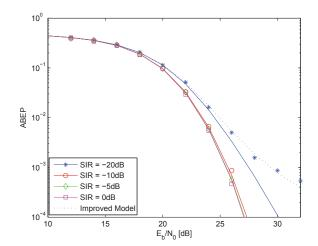
Fig. 10. ABEP of the T<sub>c</sub>-DTR receiver with 3 interferers located at  $f_{J_1} = 0.9054$ GHz (GSM band),  $f_{J_2} = 1.38105$ GHz (GNSS band), and  $f_{J_3} = 2.452$ GHz (802.11b Wi-Fi band). The "Improved Model" is given in Section IV-B. The receiver is optimized (on average) to reject the aggregate NBI (see (28)): i) C<sub>1</sub> = 0, ii)  $\sum_{j=1}^{N_s-1} c_j c_{j-1} = -31$ , and iii)  $T_c = 75.65$ ns.
