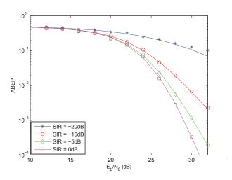
Fig. 11. ABEP of the ED receiver with 3 interferers located at  $f_{J_1}=0.9054\rm GHz$  (GSM band),  $f_{J_2}=1.38105\rm GHz$  (GNSS band), and  $f_{J_3}=2.452\rm GHz$  (802.11b Wi–Fi band).  $T_c=60\rm ns$
