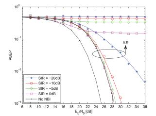
Fig. 2. ABEP of DTR and ED receivers. Solid lines: analytical model. Markers: Monte Carlo simulation. Parameter setup for DTR: i) BPAM modulation, ii)  $T_c = 60$ ns, and iii)  $T_b = N_s T_c$ . Parameter setup for ED: i) (Binary)PPM modulation, ii)  $T_c = 120$ ns, and iii) the PPM modulation shift is 60ns.
