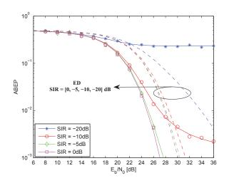
Fig. 6. ABEP of T<sub>c</sub>-DTR and ED receivers. Solid lines: analytical model. Markers: Monte Carlo simulation. As far as the T<sub>c</sub>-DTR scheme is considered, a ML code [77] with  $N_s = 63$  is considered. The ED receiver for  $N_s = 63$  is shown with dashed lines (only model).
