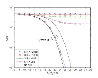
Fig. 3. ABEP of  $T_c$ -DTR and TR receivers. Solid lines: analytical model. Markers: Monte Carlo simulation. As far as the  $T_c$ -DTR scheme is considered, the optimal DS code design to meet the conditions  $C_1$  and  $C_2$  is considered. The used code is [-1, +1, -1, +1, ...]. Parameter setup for TR: i) BPAM modulation, and ii)  $T_r = 60$ ns.
