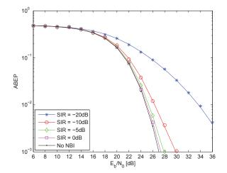
Fig. 4. ABEP of CM–TR receiver. Solid lines: analytical model. Markers: Monte Carlo simulation. Parameter setup: i) BPAM modulation, ii)  $T_c = 60$ ns, and iii)  $T_b = N_s T_c$ . Furthermore, the multiplexing codes are assumed to satisfy the condition in [12, Eq. (8)].
