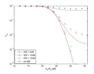
Fig. 13.  $P_m$  of the DTR receiver with 3 interferers located at  $f_{J_1} = 0.9054$ GHz (GSM band),  $f_{J_2} = 1.38105$ GHz (GNSS band), and  $f_{J_3} = 2.452$ GHz (802.11b Wi–Fi band). The receiver is optimized (on average) to reject the aggregate NBI, *i.e.*,  $T_c = 87.90$ ns.
