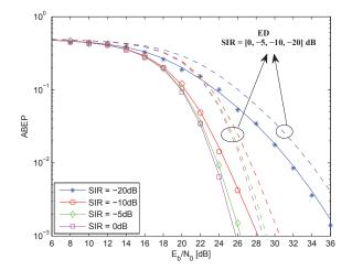
Fig. 7. ABEP of  $T_c$ -DTR receiver when  $C_1$  is verified and  $C_2$  is not, *i.e.*,  $C_1 = 0$  and  $\sum_{j=1}^{N_s-1} c_j c_{j-1} = +8$ . Solid lines: analytical model. Markers: Monte Carlo simulation. The ED receiver is shown with dashed lines (only model).
