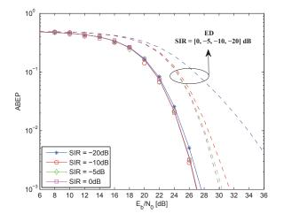
Fig. 5. ABEP of  $T_c$ -DTR and ED receivers. Solid lines: analytical model. Markers: Monte Carlo simulation. As far as the  $T_c$ -DTR scheme is considered, a Walsh-Hadamard code [77] with  $N_s = 64$  is considered. The ED receiver for  $N_s = 64$  is shown with dashed lines (only model).
