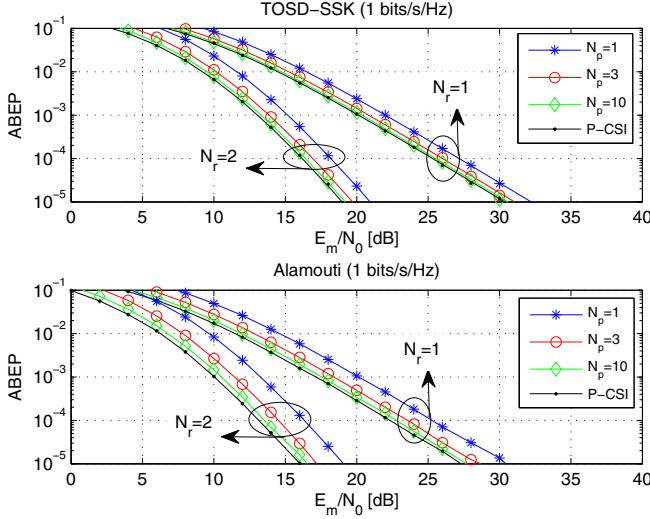
Fig. 1. ABEP against  $E_m/N_0$  for various pilot pulses  $N_p$  and rate 1 bits/s/Hz. (top) TOSD-SSK modulation: solid lines show the analytical model and markers Monte Carlo simulations. (bottom) Alamouti scheme: only Monte Carlo simulations are shown.
