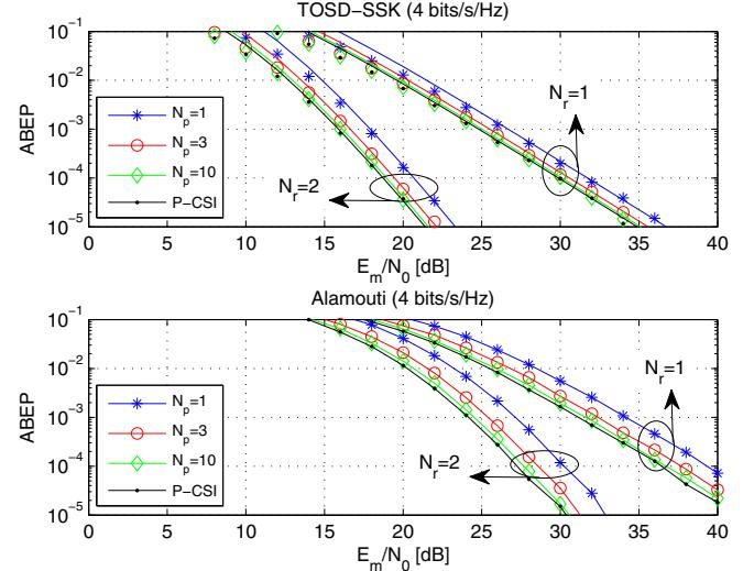
Fig. 4. ABEP against  $E_m/N_0$  for various pilot pulses  $N_p$  and rate 4 bits/s/Hz. (top) TOSD-SSK modulation: solid lines show the analytical model and markers Monte Carlo simulations. (bottom) Alamouti scheme: only Monte Carlo simulations are shown.
