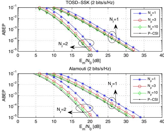
Fig. 2. ABEP against  $E_m/N_0$  for various pilot pulses  $N_p$  and rate 2 bits/s/Hz. (top) TOSD-SSK modulation: solid lines show the analytical model and markers Monte Carlo simulations. (bottom) Alamouti scheme: only Monte Carlo simulations are shown.
