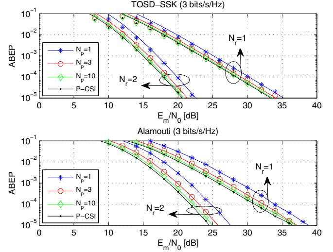
Fig. 3. ABEP against  $E_m/N_0$  for various pilot pulses  $N_p$  and rate 3 bits/s/Hz. (top) TOSD-SSK modulation: solid lines show the analytical model and markers Monte Carlo simulations. (bottom) Alamouti scheme: only Monte Carlo simulations are shown.
