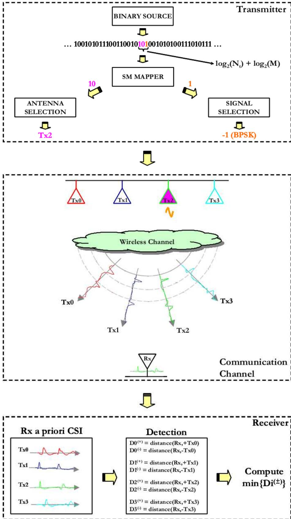
Fig. 2. SM: How it works. Setup: i)  $N_t = 4$ , ii)  $N_r = 1$ , and ii)  $M = 2$ . Legend: i) BPSK = Binary Phase Shift Keying, ii) CSI = Channel State Information, and iii)  $\text{distance}(x, y) = \text{Euclidean distance between signals } x \text{ and } y$  [7, Ref. [7]].
