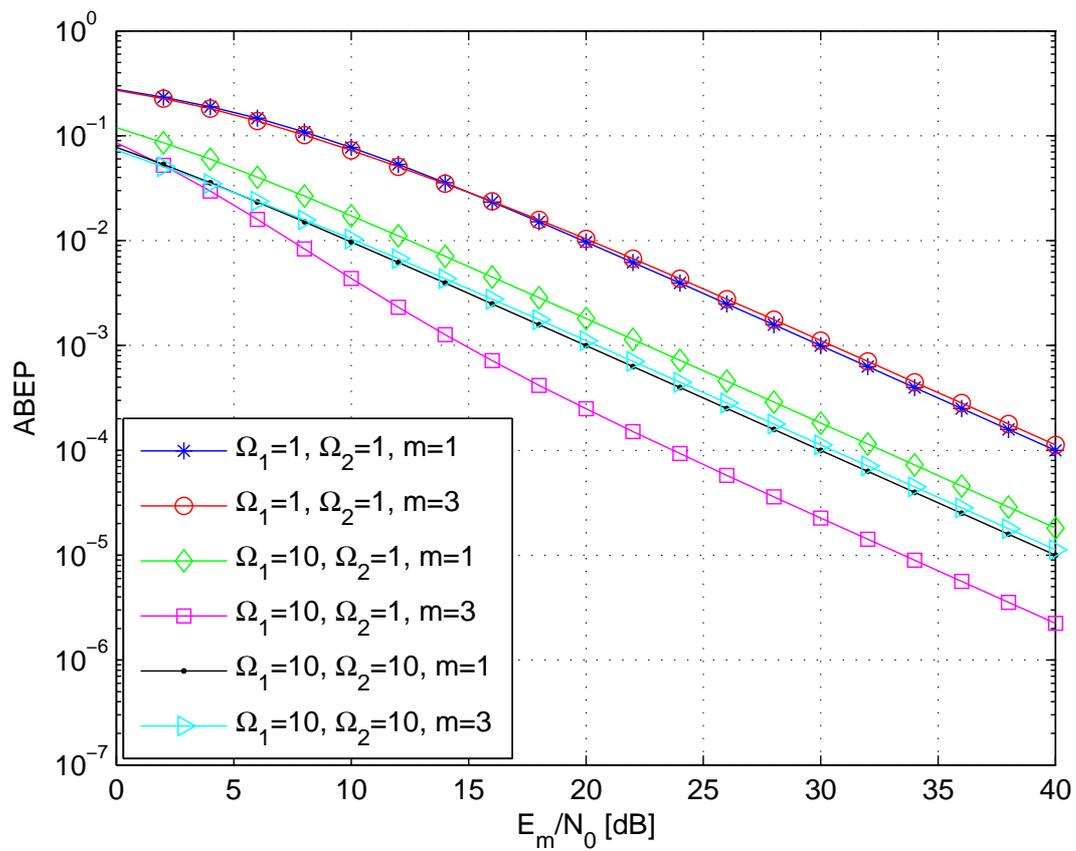
Fig. 4. Average Bit Error Probability (ABEP) against  $E_m/N_0$  for: i)  $N_t = 2$ , ii)  $N_r = 1$ , iii) uncorrelated Nakagami- $m$  fading with parameters  $(\Omega_1, m_1)$ ,  $(\Omega_2, m_2)$  [7, Ref. [7]], and iv)  $m = m_1 = m_2$ . The ML-optimum receiver in [7, Ref. [7]], [8] is considered.
