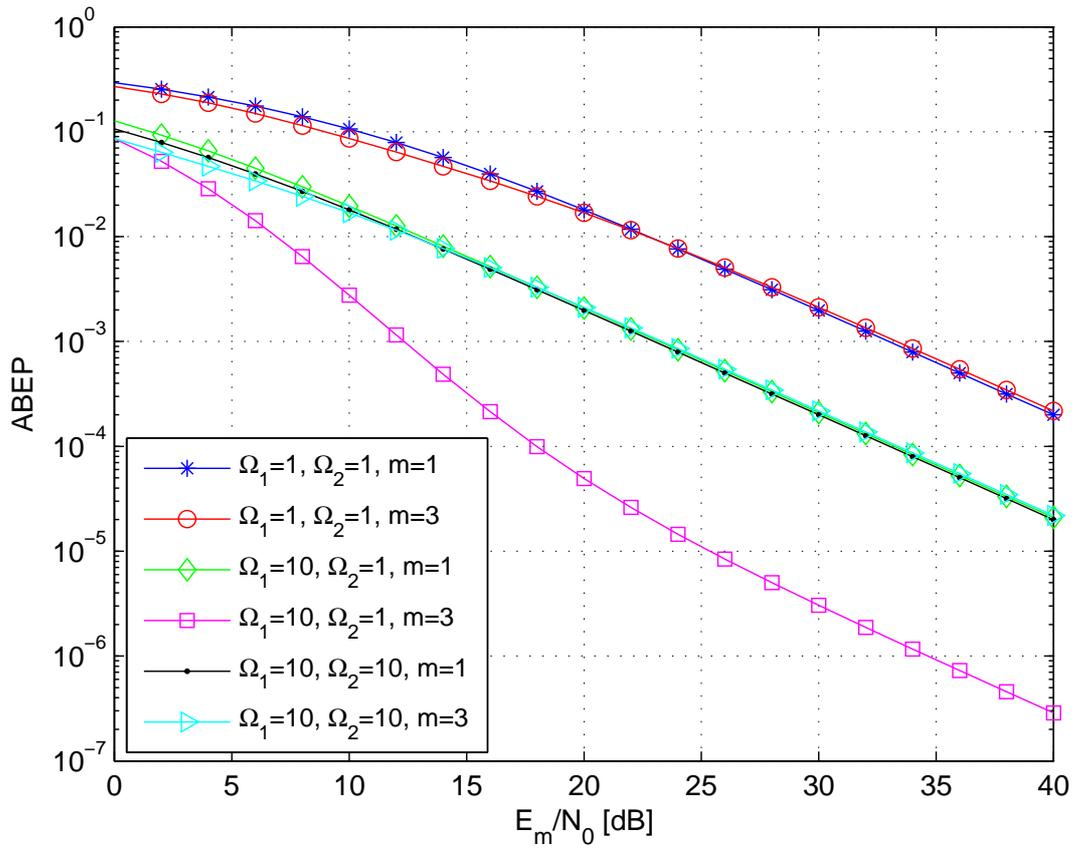
Fig. 5. Average Bit Error Probability (ABEP) against  $E_m/N_0$  for: i)  $N_t = 2$ , ii)  $N_r = 1$ , iii) correlated Nakagami- $m$  fading with parameters  $(\Omega_1, m_1)$ ,  $(\Omega_2, m_2)$  and correlation coefficient  $\rho = \rho_{1,2} = \rho_{2,1} = 0.75$  [7, Ref. [7]], and iv)  $m = m_1 = m_2$ . The ML-optimum receiver in [7, Ref. [7]], [8] is considered.
