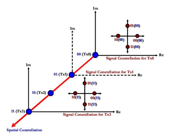
Fig. 1. Tridimensional constellation diagram of SM: each spatial–constellation point (*i.e.*, the antenna index) defines an independent complex plane of signal–constellation points. For illustration purposes, only two of such planes are shown in the figure for: i)  $N_t=4$ , and ii) M=4. Legend: i) Re = real axis of the signal–constellation diagram, and ii) Im = imaginary axis of the signal–constellation diagram.
