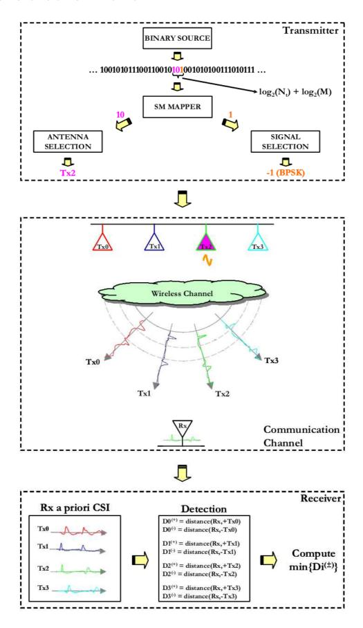
Fig. 2. SM: How it works. Setup: i)  $N_t = 4$ , ii)  $N_r = 1$ , and ii) M = 2. Legend: i) BPSK = Binary Phase Shift Keying, ii) CSI = Channel State Information, and iii) distance (x, y) = Euclidean distance between signals x and y [7, Ref. [7]].
