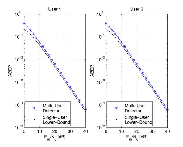
Fig. 3. Average Bit Error Probability (ABEP) against  $E_m/N_0$  for a scenario with 2 transmitters and 1 receiver (i.e., multi-user setup): i) each transmitter has  $N_t=2$ , ii) the receiver has  $N_r=1$ , iii) the channel of both users is uncorrelated and identically distributed according to a Nakagami-m distribution with parameters  $(\Omega_1, m_1)$ ,  $(\Omega_2, m_2)$  with  $m_1=m_2=1$  and  $\Omega_1=\Omega_2=1$  [7, Ref. [7]]. A multi-user ML-optimum receiver is considered [1].
