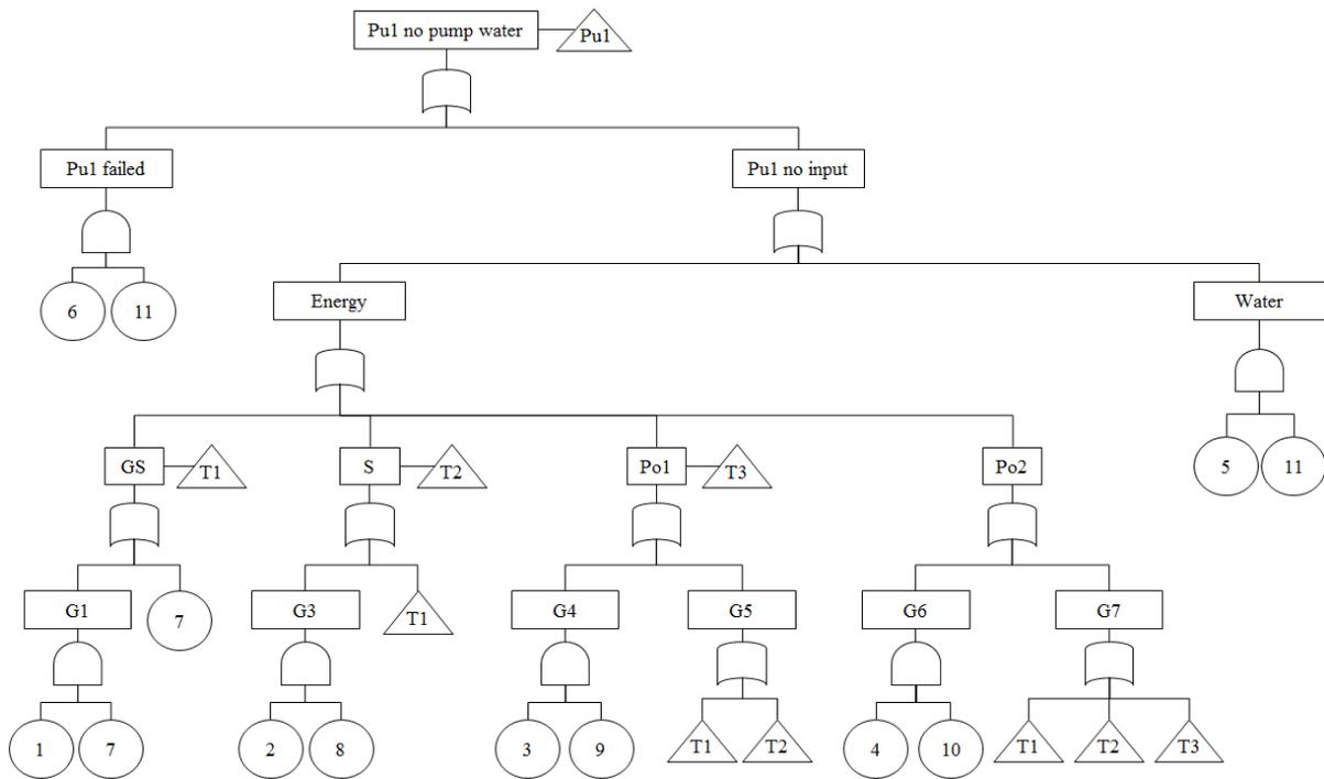
Figure 5. Fault tree details for the failure event of the component “pump” of the external water distribution system. GS: Generation Station, S: Substation, Po: Pole, Pi: Pipe, Pu: Pump, R: Road access. The numbers in the circles are referred to the failure of the components: 1→ GS, 2→ S, 3→ Po1, 4→ Po2, 5→ Pi1, 6→ Pu1, 7→ R7, 8→ R6, 9→ R5, 10→ R4, 11→ R3.
