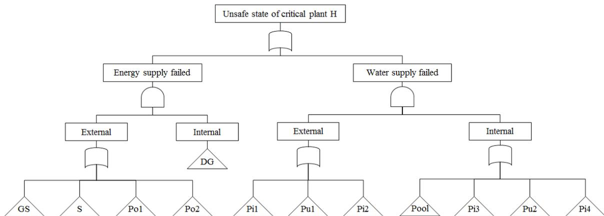
Figure 4. Fault tree of the system of systems: upper levels. The elements in the triangular shape are not detailed. NPP: Nuclear Power Plant, GS: Generation Station, S: Substation, Po: Pole, Pi: Pipe, Pu: Pump, DG: Diesel Generator.
