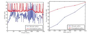
**Fig. 2.** Evolution of the PSNR as a function of time (left) and of the channel rate (right) for the forman qcif sequence when  $\pi_{\rm m}^*(\mathbf{s})$  and  $\pi_{\rm f}^*(\mathbf{s})$  are applied
