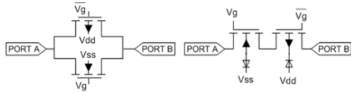
Figure 4. Conventional switch (left) and in-series switch (right) [18]
