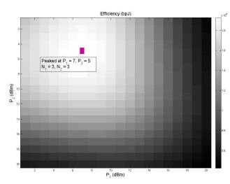
Fig. 3.  $\eta$  over combinations of  $P_1$  and  $P_2$  with  $\frac{b}{\sigma^2} = 100$  (20dB),  $N_1 = N_2 = 3$ . As before, zone 2 corresponds to a lower SINR and interestingly, in this case, the efficiency is optimized by using more power along the zone 1 user. This is because with 3 users in each zone, the demanded rate exceeds the maximum available throughput and so, optimization is done by using power on users with a better SINR.
