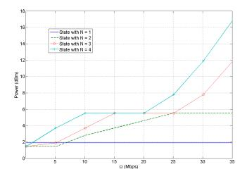
Fig. 4. The power allocation scheme  $(P_1, \dots, P_4)$  plotted against the traffic  $\Omega$  when  $\hat{\eta}$  is optimized. Also note that the QoS constraint of maintaining the blocking rate below 0.01 is satisfied.
