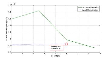
Fig. 6.  $\hat{\eta}$  plotted against the traffic  $\Omega_1 = \lambda_1 S$  when  $\hat{\eta}$  is optimized and when  $\eta$  is optimized for each state separately. Also note that the QoS constraint of maintaining the blocking rate below 0.01 is satisfied at all points shown.
