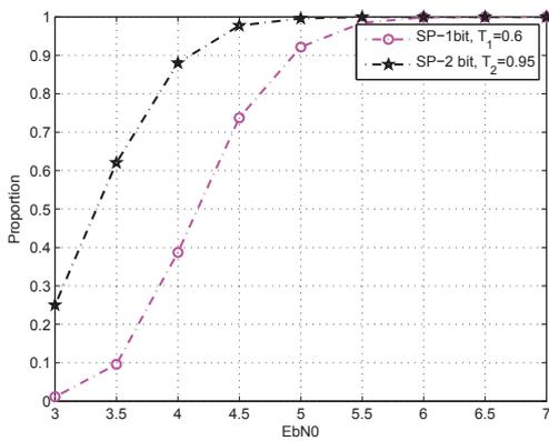
Fig. 5. Proportion of frames above threshold vs  $E_b/N_0$
