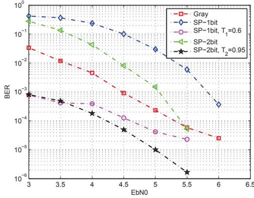
Fig. 4. BER versus  $E_b/N_0$  over AWGN channel
