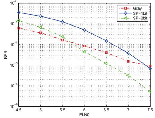
Fig. 6. BER versus  $E_b/N_0$  over fading channel
