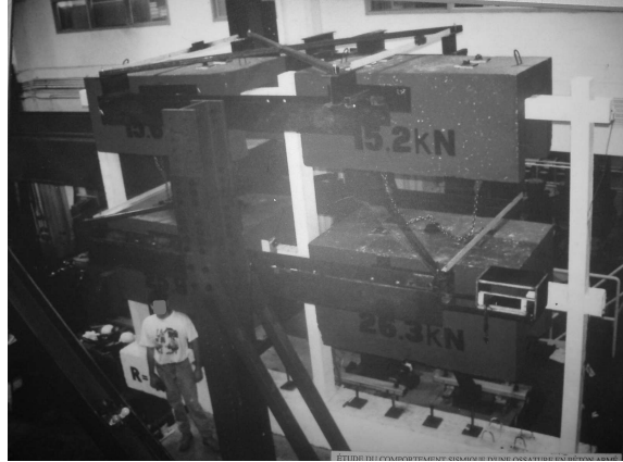
Figure 1: RC frame structure tested on the shaking table at École Polytechnique in Montreal. Dimensions are in [mm].
