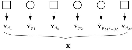
**Fig. 1** Example of NLA and its equivalent VULA, with  $\mathbf{d} = [0, 2, 5] \frac{\lambda}{2}$ ,  $\mathbf{p} = [1, 3, 4] \frac{\lambda}{2}$  and  $\mathbf{g} = [1, 0, 1, 0, 0, 1]$ .  $\square$ : existing sensors ( $\mathbf{Y}$ ),  $\circ$ : omitted sensors ( $\hat{\mathbf{Y}}_{\mathbf{p}}$ ).
