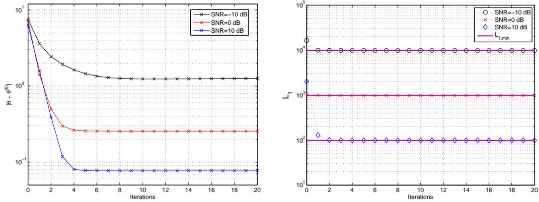
**Fig. 8** RMSE of the source at  $10^\circ$  for the nonregular array  $\mathbf{d} = [0, 1.32, 3.03, 5] \frac{\lambda}{2}$ , at SNR = -10, 0 and 10 dB,  $DOA = [-5^\circ, 10^\circ]$ . **Fig. 9** Negative log-likelihood for the nonregular array  $\mathbf{d} = [0, 1.32, 3.03, 5] \frac{\lambda}{2}$ , at SNR = -10, 0 and 10 dB,  $DOA = [-5^\circ, 10^\circ]$ .
