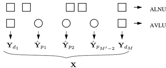
**Fig. 2** Example of a nonregular array and its equivalent VULA, with  $\mathbf{g} = [1, 0, 0, 0, 1]$ . In the VULA,  $\square$ : existing sensors ( $\mathbf{Y}$ ),  $\circ$ : omitted sensors ( $\hat{\mathbf{Y}}_{\mathbf{p}}$ ).
