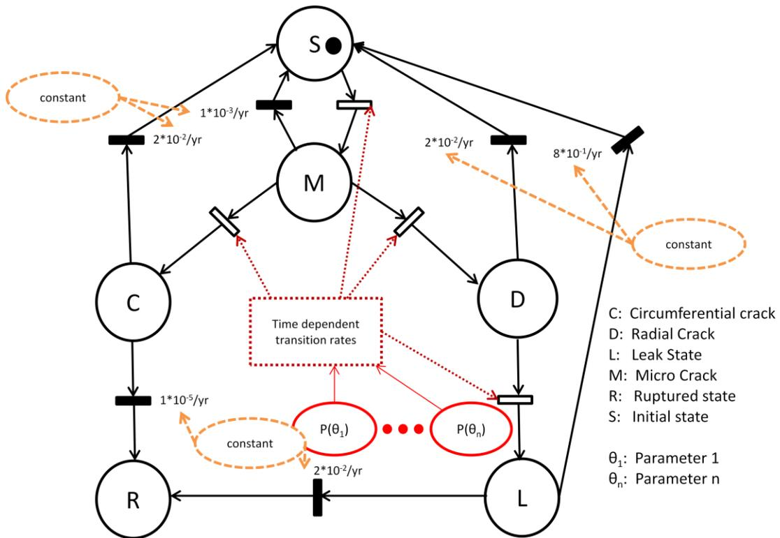
Fig 4. The SPN simulation model of Alloy 82/182 dissimilar metal weld degradation.
