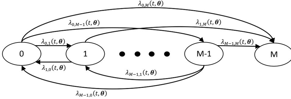
Fig 1. A State-space diagram of the component degradation process.
