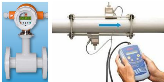
Figure 2. On the left: standard commercial electromagnetic flow meter; on the right: measuring flow rates with an ultrasound flow meter.
